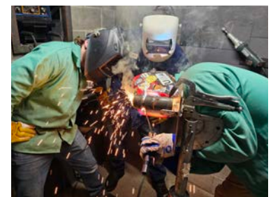
Instructor Matt Ruggles demonstrates an efficient uphill welding technique in the 5G position to student participants.
