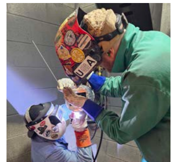
Instructor Matt Ruggles observes the root penetration of the weld bead through a dark lens, rated for viewing the welding arc, to provide real-time guidance and feedback to the student participant.
